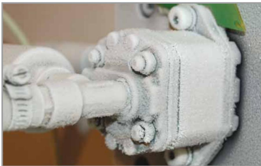
FIG. 1 Marzocchi K0.5 Gear pump on cold-start test at -45°C
